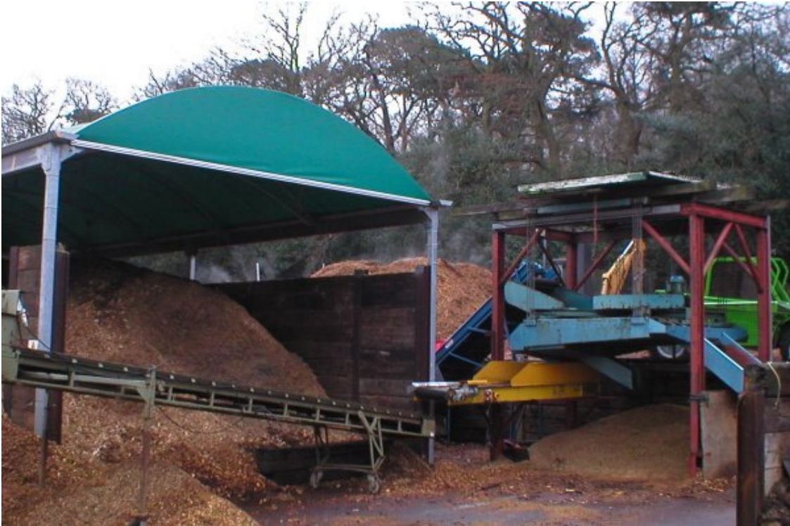
Picture 8: Wood Chip Production for Slough Heat & Power at Croydon's tree station
